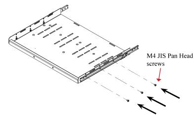
**Step 6 Install left inner rail.** Repeat same step as STEP 5 for the left side.
