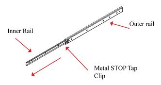
**Step 2 Installing Sliding Rail Ear Brackets.** Slide the rear ear bracket to desire depth. Align the first mounting hole from the right with thread ed hole on the rear ear bracket. If unable to align with a threaded hole, use included K-Lock Nuts to secure M4 screw instead.
